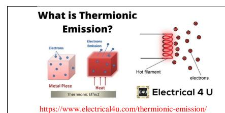
Thermionic emission is the **emission of electrons from a heated metal (cathode)**. As the temperature increases, the surface electrons gain energy. The energy acquired by the surface electrons allows them to move a short distance off the surface thus resulting in emission.
