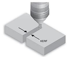
When talking about CNC shape cutting with typical cutting processes, kerf is the width of material that the process removes as it cuts through the plate.
