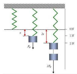
Diagram of Hooke's Law: The extension of the spring is linearly proportional to the force.
