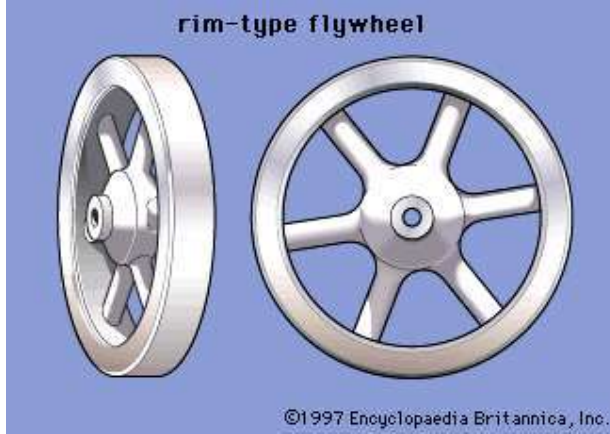
(A) rim-type flywheel; (B) tapered-disk flywheel Encyclopaedia Britannica, Inc.
